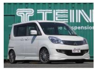
\*For vehicles manufactured on or after January 1st, 2006, if the lower edge of the fog light is less than 250mm from the ground when lowered, it may not comply with Japan's vehicle safety regulations. Please adjust the ride height to secure the minimum 250mm clearance. For details on inspection standards, please contact the nearest National Agency of Vehicle Inspection.
